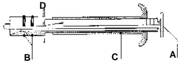
2) Slide the two (2) 3/4" O-rings onto the bottom of the gravity feed tube until they drop in the O-rings grooves.
